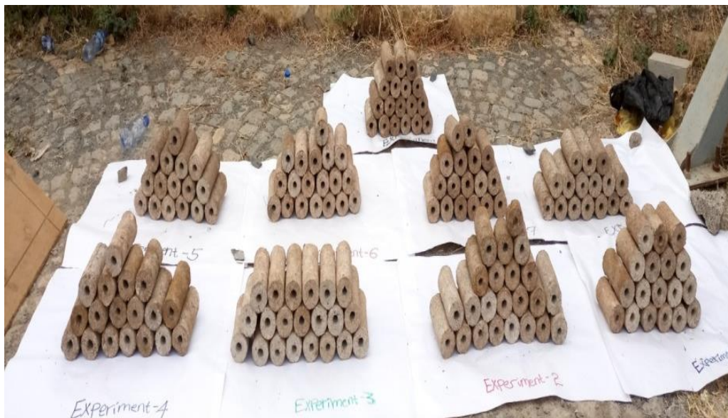
Figure 4: Briquettes from nine experiments on open-sun drying
