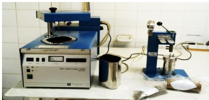
Figure 2: Bomb calorimeter used in mesebo cement factory
